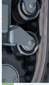
▲ Fixed rollers for excellent stability
